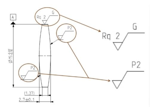
The ISO standard allows to define this parameter more exactly. In many cases this is level of detail may not be required, but in some applications **surface texture** is crucial. Look at the picture below.
