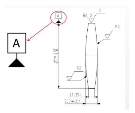
The key function of the **datum surface** is to define "reference point" for all other geometrical requirements for the lens (or for another mechanical or optical element which was drawn on the drawing).
